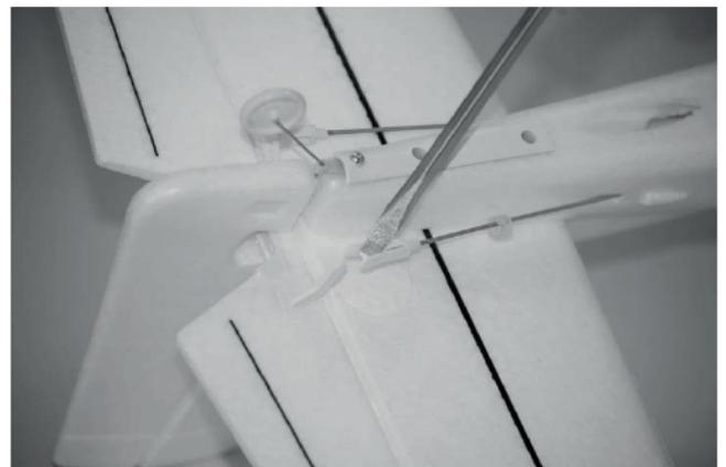
After connecting both clevises with the control horns, take a straight look from above onto the rudder. It should be in line with the tailplane. If the rudder tilts left or right, you can adjust the position of the clevis / pushrod to center it while the trim lever remains centered.
