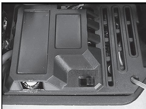
2. Plug the ESC to the battery cable to switch ESC on.
