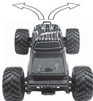
4. Rotate the wheel counter-clockwise to turn left. Rotate the wheel clockwise to turn right.
