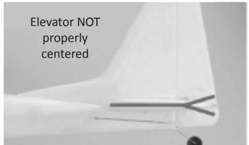
Observe the elevator to ensure it is properly centered as shown above.
