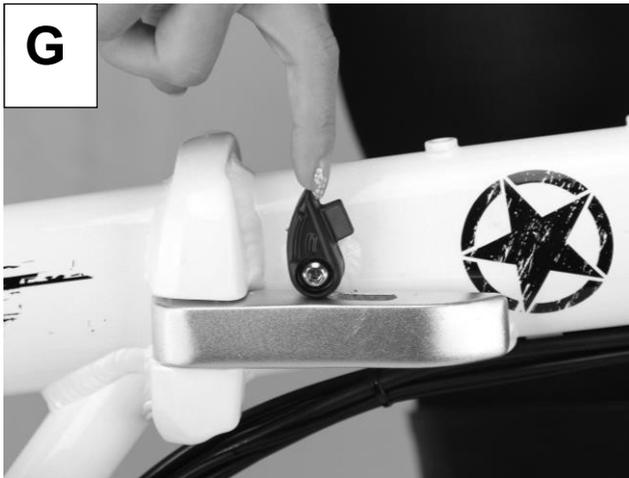
5. To fold bicycle frame, move the frame safety hook to the open position (see photo called G) and open the safety latch lever of the frame.
