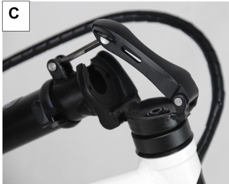
Fold down the stem and adjust the position of T-handle: ensure the front wheel stays parallel to the handlebar (see below photo called D).
