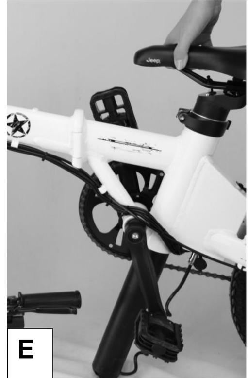
4. Adjust the left crank angle to the 9 o'clock direction (left crank is pointed forward and downward at a 45° angle). See photo called F.
