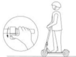
3, Step on the other leg when the scooter is moving, then press the accelerate button (only accelerate when the scooter speed is beyond 5km/h)
