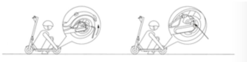
If you feel the brakes are too tight, use the M5 hex wrench counterclockwise to release the plate screws on the disc, slightly shorten the tail brakes cable then lock it up with plate screws; If you feel the brakes are too loose, release the plate screws and slightly extend the tail brakes cable to the tail side and tighten the screws again.
