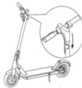
3 Use the hex wrench in the packing box to lock the screws on both sides
