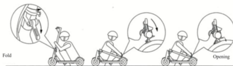
Make sure the scooter is off and open the folding wrench in the front bar like picture showing above. Dip down the front bar to the hook in the rear fender and tie it up. When you want to use it the scooter again, just simply release the hook and lift the front bar up and lock the wrench again.
