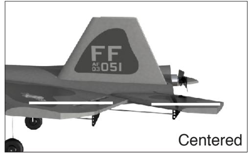
Observe the hinges to ensure it is properly centered as shown on the right.
