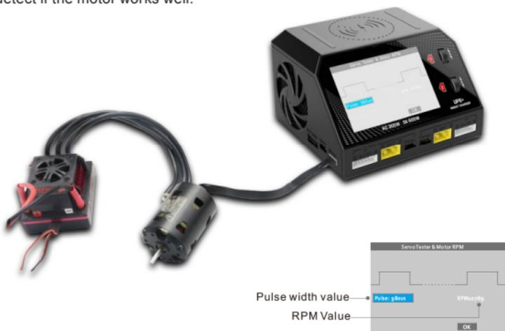
Servo testing: By adjusting and changing the pulse width, it can be detected if the servo's direction and angle are normal.
