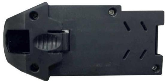
This model is equipped with a pluggable camera which can be pulled out through pushing the locking knob.
