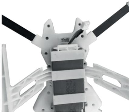
Put the battery into the mounting on the bottom of the model.
